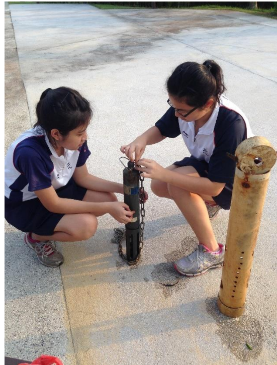
Figure 2.12 NIE student on overseas field course measuring the Secchi depth in the Buffalo River, New York (left) and NIE student using a Secchi tube at Jurong Ecogarden (right THIS PHOTO WILL CHANGE!!!!!!!!!! ).
