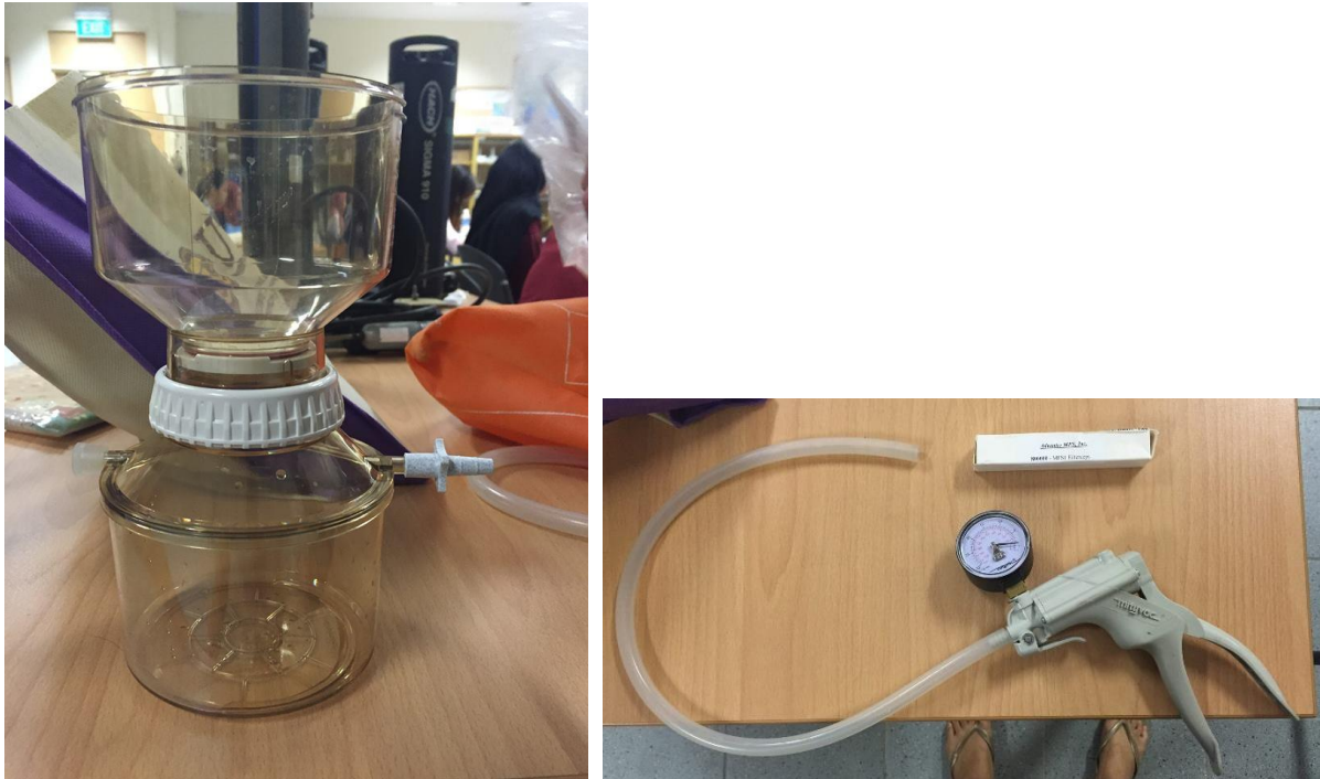
Figure A5 Filter holder system (left) and hand operated vacuum pump that attaches to the filter holder system (right) to help draw the sample through the filter (photos courtesy of Zee Wan Teng).
