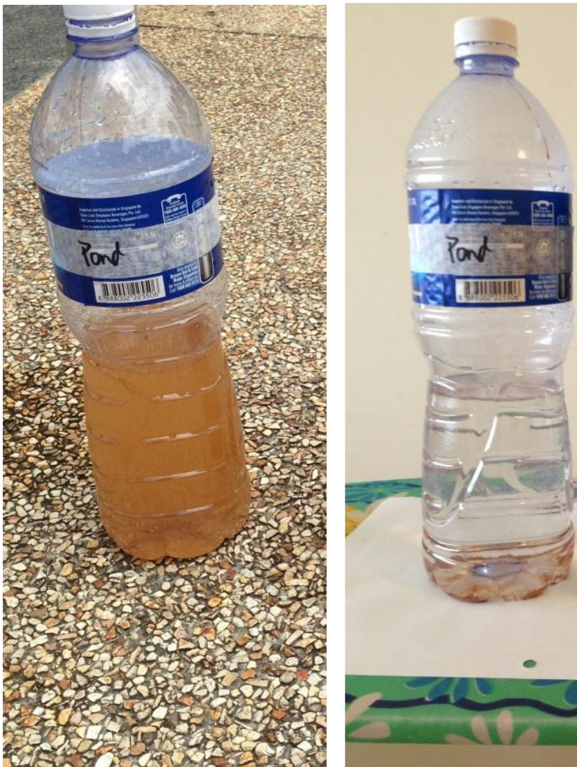
Figure 2.15 Admiralty Park stormwater pond waters immediately after sampling (left) and after a two day hold time (right).
