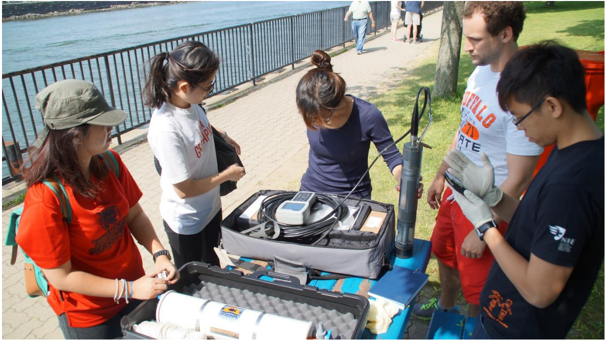
Figure 5.5 Preparing the YSI 6920 datasonde to be lowered into the Buffalo River.
