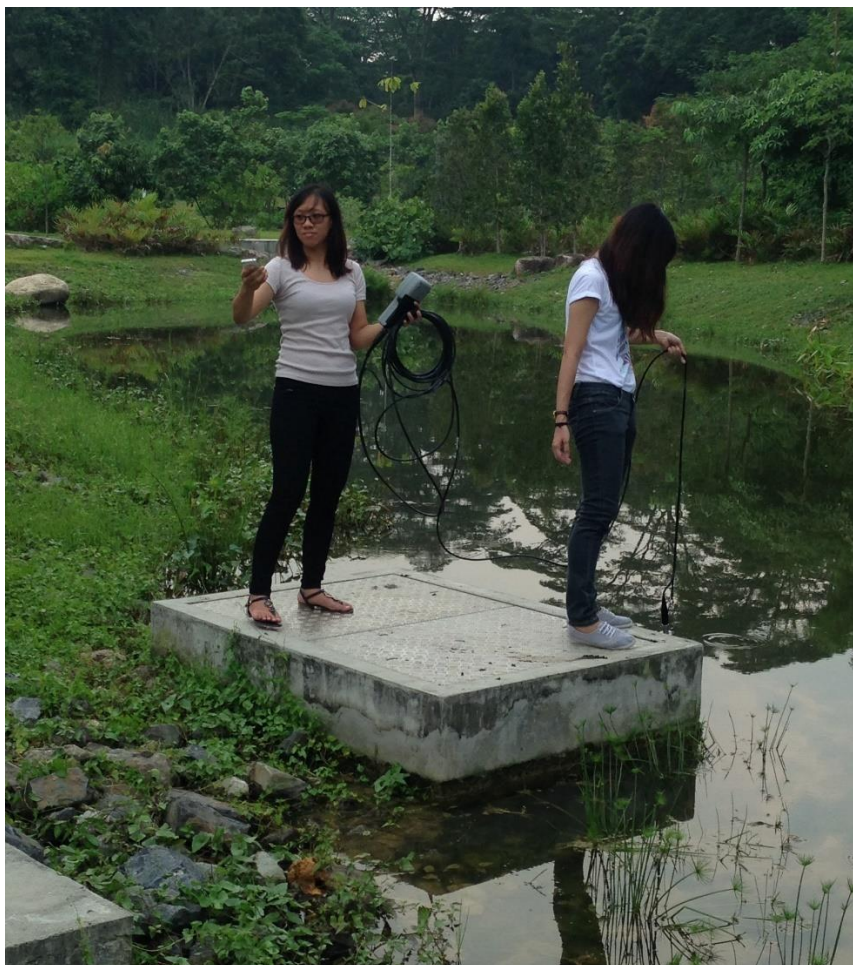
Figure 2.1 (a) Dissolved oxygen levels logged at 15 minute time steps using a YSI 6920 datasonde in the Jurong Ecogarden pond upstream of the biotope; and (b) NIE students manual sampling with the YSI 6920 datasonde at the location where it was installed upstream of the biotope for the data logging.
