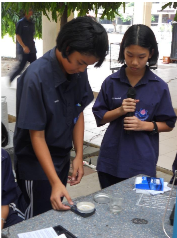
Figure A4 M3 students from Kanaratbamrung Pathumthani school, Thailand, measuring total solids in an aluminum evaporation dish, using a small portable electronic balance (left) and an example sample from the Chao Phraya River (right).
