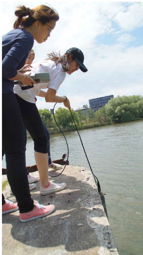
Figure 5.6 Lowering the YSI 6920 into the Buffalo River AOC.
