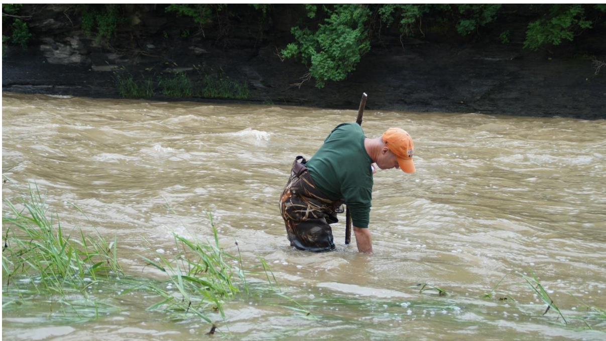
Figure 5.4 Collecting manual grab samples during a storm event. Safety must be the top priority, so the heavier, more experienced professor lends a hand in sample collection on this day. Note that it is important to stand downstream of the sample collection point to avoid contaminating the sample.
