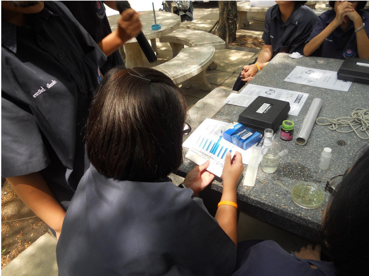
Figure A1 An M3 student from Kanaratbamrung Pathumthani school, Thailand, comparing the color standards to determine dissolved oxygen level in a sample from the Chao Phraya River.
